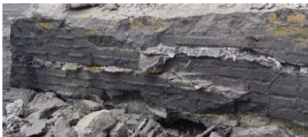
Fig. 5. Metal infiltrations in the horizontal cracks of a domestic cathode
