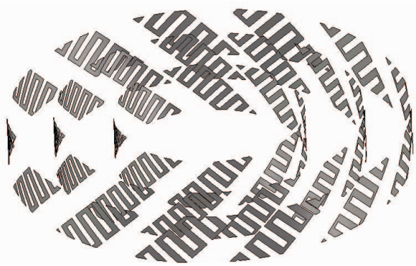
Fig. 9. Segment of 3-layer polarizer structure.
