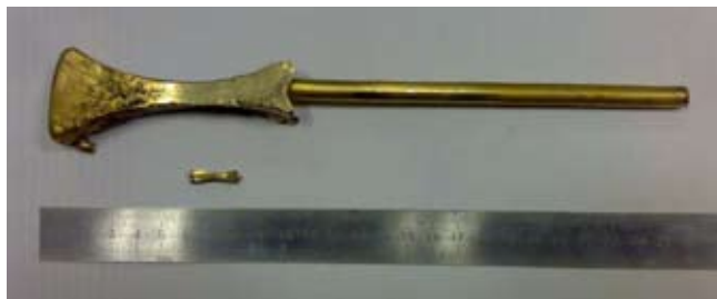
Fig. 6. Press residues and press products obtained by the combined treatment of alloy SAg-40 in different experimental setups
