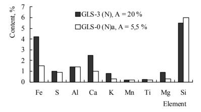
Fig. 7. Element composition of graphite GLS-3 (N) (A - ash content)
