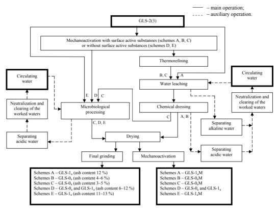
Fig. 16. Schemes of dressing cryptocrystalline graphites
