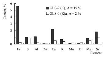
Fig. 8. Element composition of graphite GLS-2 (K) (A - ash content)
