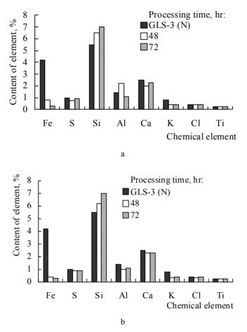
Fig. 14. Dependence of the element composition of the ash admixtures of Noginsk graphite GLS-3 (N), on the time and temperature of processing (a - 20 °C; b - 80 °C)
