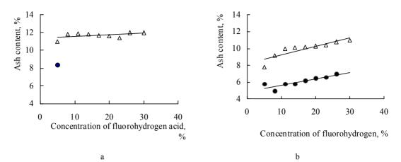
Fig. 6. Dependence of the ash content of non-activated graphite and activated graphite GLS-3 (N) on the concentration and temperature of the fluorodydrogen acid: a – initial graphite; b – activated graphite;  $\Delta$  – without heating;  $\bullet$  – with heating
