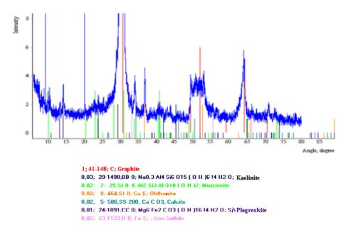
Fig. 11. Phase composition of graphite GLS-2 (K)
