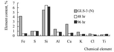
Fig. 15. Dependence of the element composition of graphite GLS-0 (N)a on the processing time
