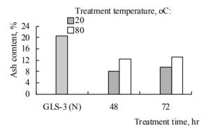
Fig. 13. Influence of microbiological treatment temperature on the ash content of graphite GLS-3 (N)
