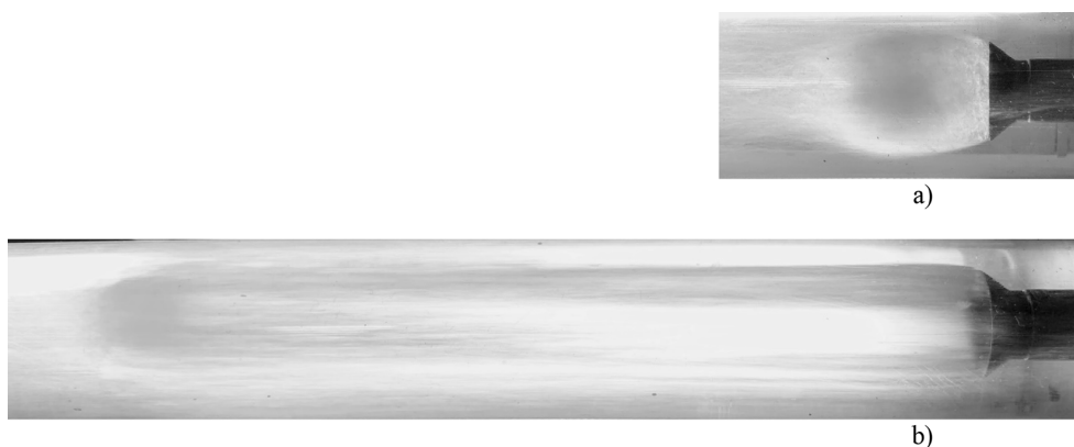
Fig. 5. An example of the geometry of a cavern when flowing around a cone with a diameter of 15.45: a – the length of the cavern is 30 mm; b – the length of the cavern is 220 mm
