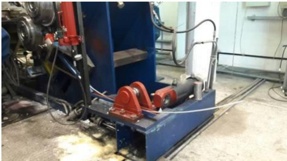
Picture 3.1 – General view of extrusion block of combined processing plant with an extruded rod.
