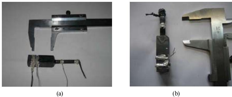
Fig. 3. The appearance of contact assemblages after 10 (a) and 100h (b) holdings at 900 °C and 20A load
