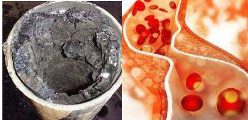
Figure 1 - Pipeline diameter reduced by asphaltene agglomeration thus reducing oil flow in the pipeline (left) and Coronary artery diameter reduced/almost blocked by plaque formed from cholesterol thus reducing blood flow (right).
