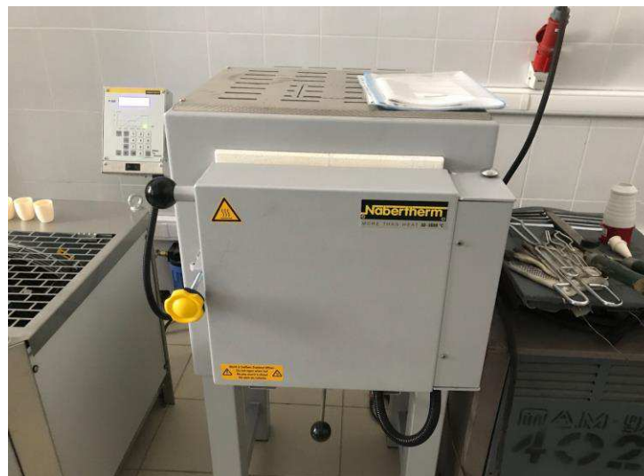
Figure 20-Nabertherm Oven (temperature range 30-3000°C)
