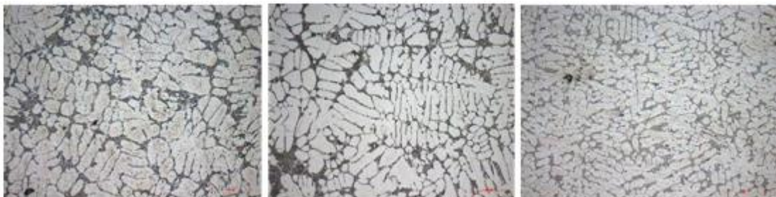
Figure 5. Microstructures and sizes of dendritic cells at the periphery of the samples, x 200: a) sample P1 - 16.8 microns; b) sample P3 - 13.1 \mu m ; c) sample P4 - 11.3 \mu m .
