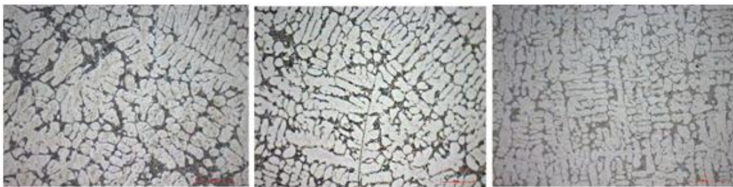
Figure 4. Microstructures and sizes of dendritic cells in the middle of the samples.
