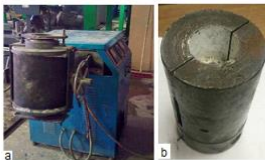
Figure 1. Melting equipment: a - Tamman furnace; b - chill mold.
