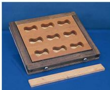
Figure 2. A core box with a rail for cutting off excess mixture.
