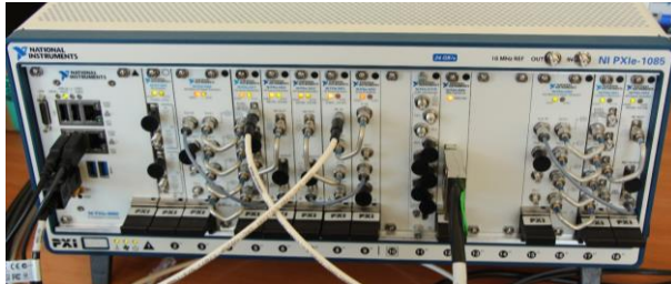
Figure 5. Appearance of the generator based on the PXIe National Instruments chassis.
