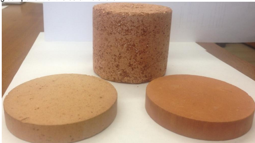
Figure 6. The appearance of ceramics with additives of expanded vermiculite in different ratios in comparison with the control sample
