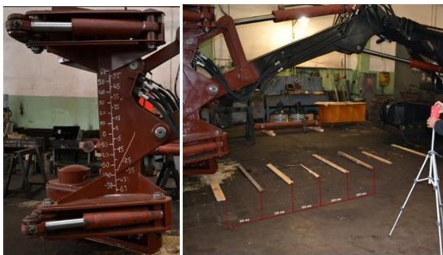
Figure 8. Schemes for applying a vertical and horizontal measuring scale.
