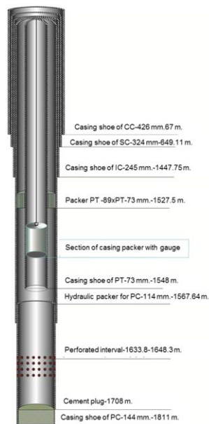
Figure 11—Schematic layout of the hydrodynamic research downhole equipment, involving the closure of the well at the bottom (casing packer).
