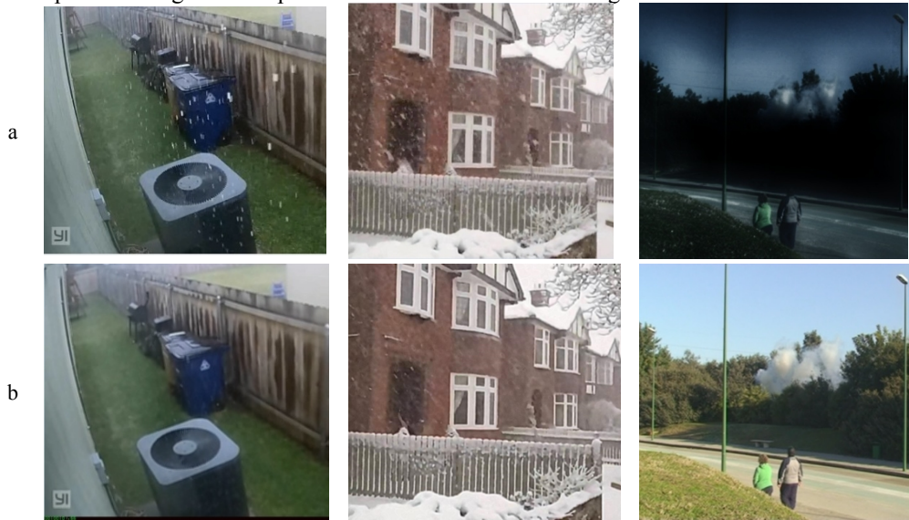
Fig. 3. Compensation algorithm experimental results: a - weather effects; b – artifacts is removed
