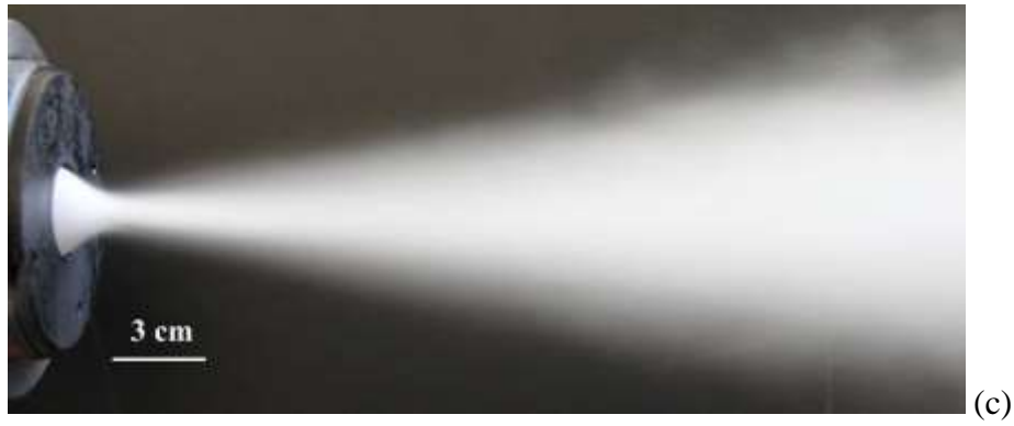
Fig. 6. Visualization of the gas-droplet flow for different values of excess pressure: (a) P_0 = 1 bar; (b) P_0 = 2 bar; (c) P_0 = 3 bar.
