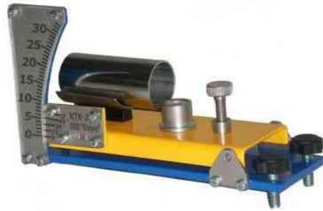
Figure 2. CFC-2 device for measuring the friction coefficient of filter cake.
