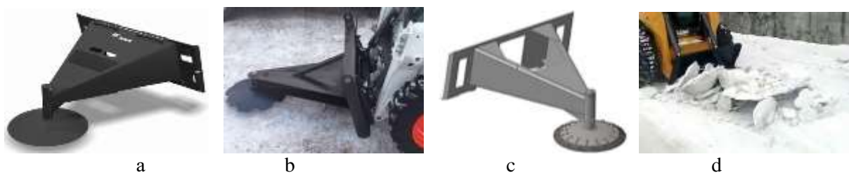
Figure 4. Bobcat Scraper: a – Bobcat scraper with a round disk; b – Bobcat scraper with a disk with semicircular cutouts along the perimeter; c – ice cleaver with replaceable cutters; d – destruction of strong snow–ice formations with a scraper.
