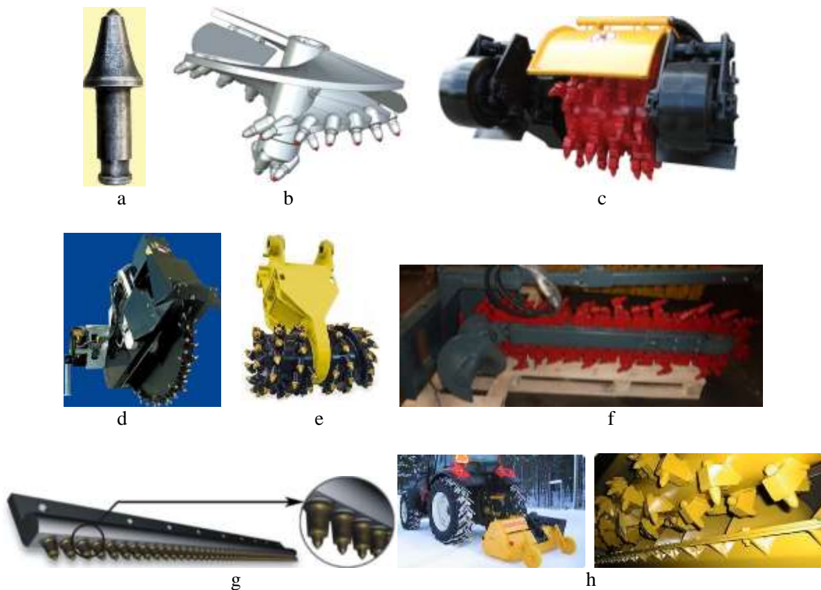
Figure 1. The use of rotary cutters in the working bodies of drilling and earthmoving machines: a – rotary cutter; b – drill cone; c – road cutter; d – milling trencher; e – milling and loosening equipment; f – chain trencher; g – blade grader; h – ice breaker SASNOMAC KT-2.
