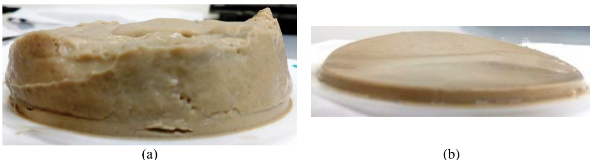
Figure 6. Photos of filter cake for a base mud with an AlN of 0.5 wt.% to (a) and after (b) the addition of SiO 2 2 wt.%.
