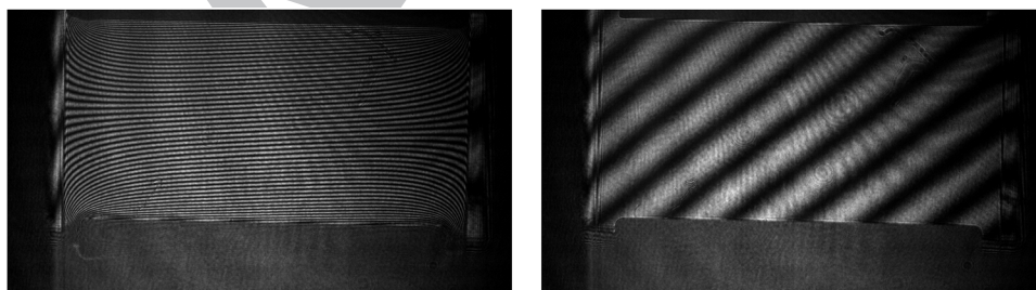
FIG. 5. Comparison of typical interference patterns. Left: pattern recorded during the Soret phase of an experimental run. Right: pattern recorded during the diffusion phase.
