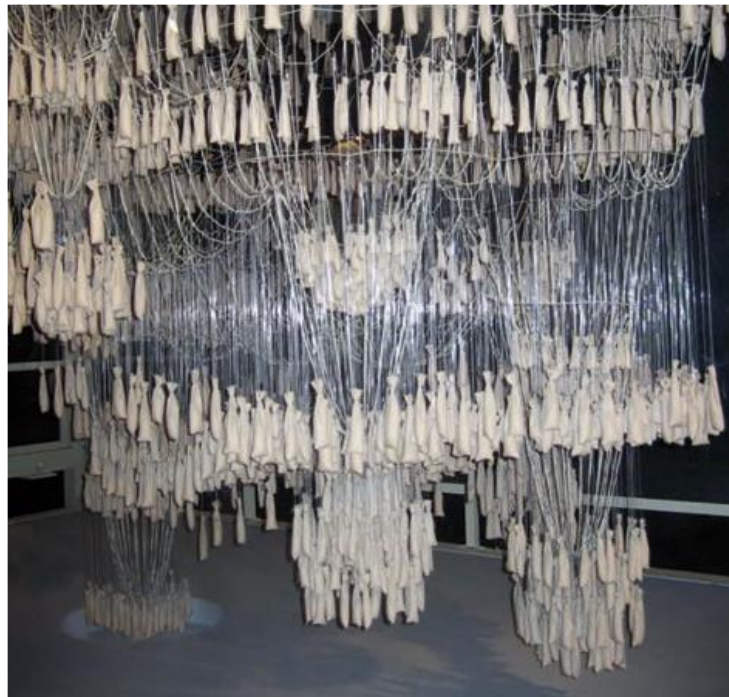
Figure 1. Reproduction of Gaudí’s hanging model for the crypt of Colònia Güell, Barcelona
