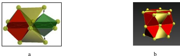
Fig. 4. Cluster model of the transition from the structure with the bcc lattice to the hcp lattice through the fcc phase
