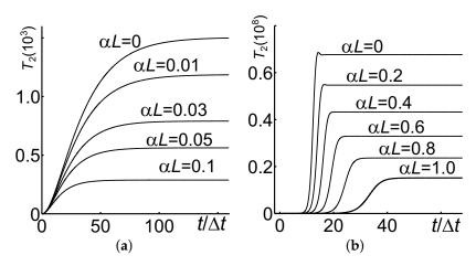
**Figure 14.** Effect of absorption on the transients in the optical parametric amplification for two different intensities of the pump field.  $-v_1=v_2=v_3=v$ .  $\alpha_1=\alpha_2=\alpha_3=\alpha$ . (a)  $gL=0.984\pi/2$ ; (b)  $gL=1.3\pi/2$ .
