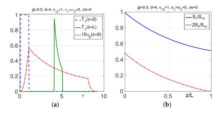
**Figure 7.** Backward-wave second harmonic generation: the effect of pulse width. Here, the input pulse duration is decreased four times as compared with Figure 6a at the same peak intensity. (a)  $T_1$  is the pulse shape for the fundamental radiation, and  $\eta_2$  is for the second harmonic; (b)  $S_1(z)$  is the fundamental pulse energy,  $S_{10} = S_1(z=0)$ ,  $2S_2/S_{10}$  is the energy (photon) conversion efficiency per pulse, and d = L/l = 4.
