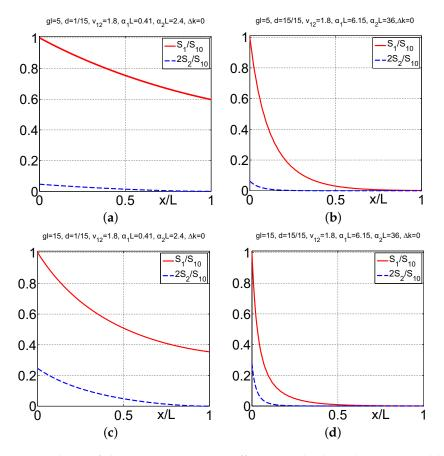
**Figure 8.** Dependence of the energy conversion efficiency at backward-wave second harmonic generation on the metaslab thickness, intensity, and duration of the pump pulse. (**a**,**b**) gl = 5; (**c**,**d**) gl = 15; (**a**,**c**) L/l = 1/15; (**a**,**d**) L/l = 1.
