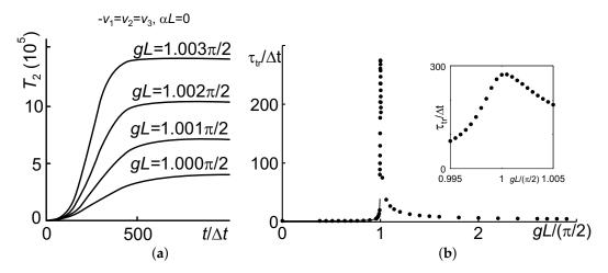
**Figure 13.** (a) The shape of the signal forefront in a transparent material at pump intensities above the critical input value  $gL = \pi/2$ ; (b) dependence of the transient period  $\tau_{tr}$  on the maximum intensity of the pump field.  $-v_1 = v_2 = v_3 = v$ ,  $\alpha_i = 0$ .
