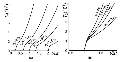
**Figure 16.** Dependence of the transient processes in three-wave mixing on the forefront of the output pulses on the dispersion of the group velocities of the coupled waves.  $gL = 0.996\pi/2$ ,  $\alpha_j = 0$ . (a)  $-v_1 = v_3$ ; (b)  $v_2 = v_3$ .
