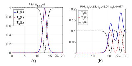
**Figure 20.** Output fields vs. intensity of the pump for the ordinary, co-propagating coupling scheme. (a) Attenuation-free material; (b) effect of attenuation dispersion. All attenuation parameters are the same as in Figure 18 (a,b), respectively.
