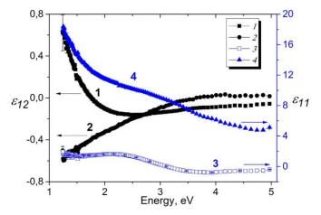
Fig. 3. The calculated values of real and imaginary parts of the Fe diagonal  $\epsilon_{11}$  and off-diagonal  $\epsilon_{12}$  dielectric permittivity tensor elements:  $1 - \epsilon'' 12, 2 - \epsilon' 12, 3 - \epsilon' 11, 4 - \epsilon'' 11$ .
