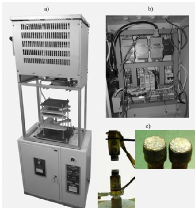
Fig. 2. The elements of the laboratory equipment for measuring the erosion wear of contact materials: a – the main frame of the bench, b – the control block, c – the element of the device for fastening and moving the contact tips and view of a contact surface after testing
