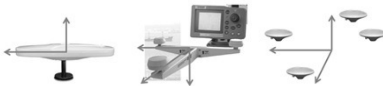
Fig. 1. Measuring axes of two, three and four antennas of ANR
