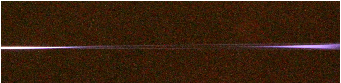
Fig. 4. Photo of filamentation area under aberration focusing by mirror. Light propagation from left to right. Bright regions are geometrical foci. Plasma formation between two thick beams in second foci region is an energetic reservoir
