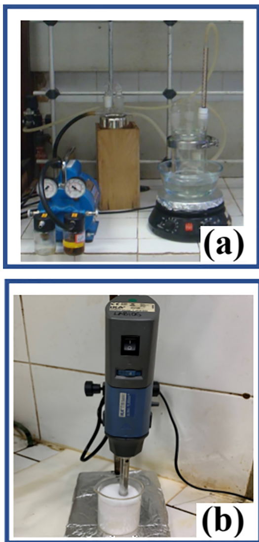
Fig. 4. System used for polymer synthesis (a) and emulsion process used in the production of polymer spheres containing the drug (b)
