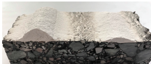
Fig. 4. Coating tracks sprayed at an air stagnation temperature of 160 (left) and 26 °C (right)
