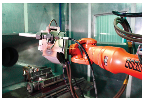
Fig. 2. Cold spray unit on industrial robot
