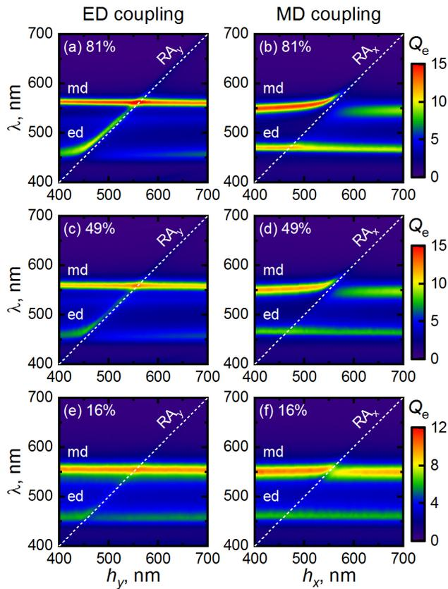
**Fig. 9.** Extinction spectra  $Q_e$  for quasi-random 2D lattices, as shown in Fig 3(d), for different number of NPs: (a)-(b) 81% = 729, (c)-(d) 49% = 441, and (e)-(f) 16% = 144 kept untouched in  $N = 30 \times 30$  arrays of NPs with  $R = 65$  nm. Note the different color scale in the last row (e)-(f).
