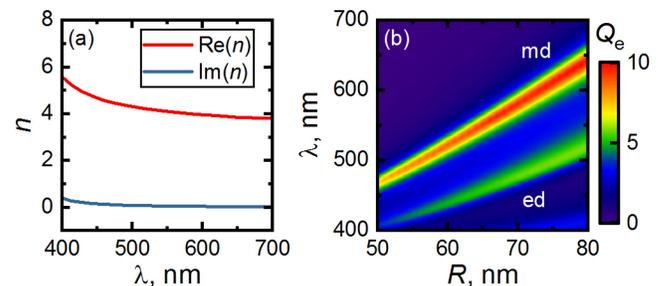
**Fig. 1.** (a) Refractive index  $n$  of Si from Ref. [87]; (b) Extinction spectra for a single Si NP of various radii  $R$  taking into account high-order multipoles. Spectral positions of electric and magnetic dipole resonances are denoted as 'ed' and 'md', respectively.
