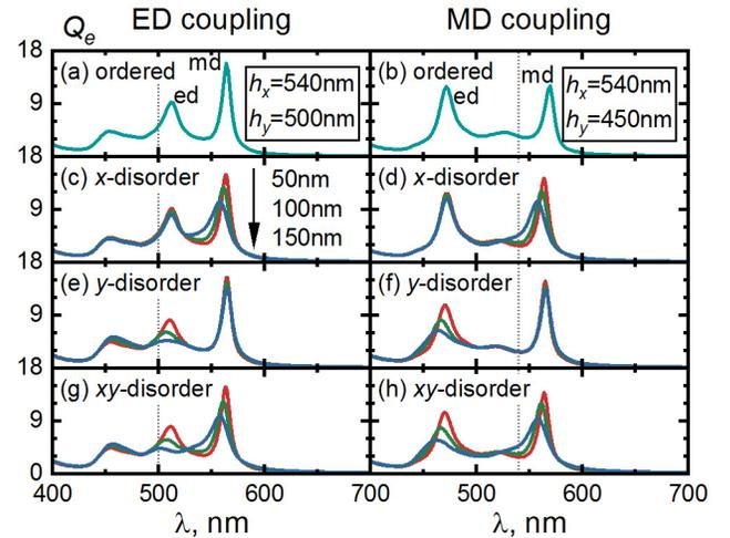
**Fig. 6.** Extinction spectra  $Q_e$  of NPs arrays with ED coupling (left), and MD coupling (right) for various degrees of positional disorder  $\sigma_x$  (c,d),  $\sigma_y$  (e,f), and  $\sigma_{xy}$  (g,h). Corresponding values of  $h_x$  and  $h_y$  are shown in legends. Dashed vertical lines denote positions of Rayleigh anomalies  $RA_y$  at  $\lambda = 500$  nm (left), and  $RA_x$  at  $\lambda = 540$  nm (right).
