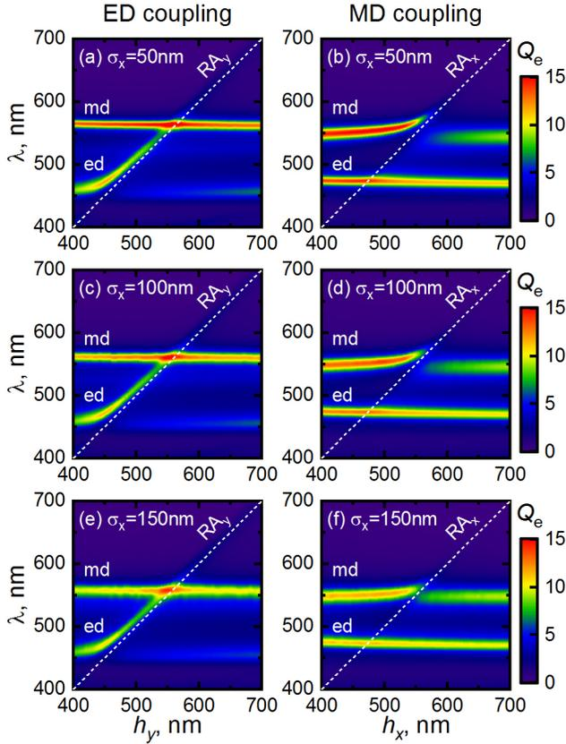
**Fig. 4.** Extinction spectra  $Q_e$  for the same 2D lattices as in Figs. 2(c) and 2(d), but for various degrees of positional disorder  $\sigma_x$  along  $x$  axis, as shown in Fig 3(a).
