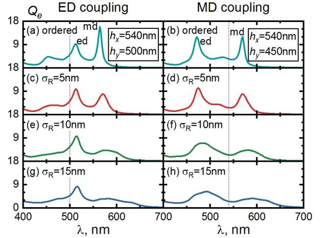
**Fig. 8.** Extinction spectra  $Q_e$  of NPs arrays with ED coupling (left), and MD coupling (right) for various degrees of size disorder  $\sigma_R$ . Corresponding values of  $h_x$  and  $h_y$  are shown in legends. Dashed vertical lines denote positions of Rayleigh anomalies  $RA_y$  at  $\lambda = 500$  nm (left), and  $RA_x$  at  $\lambda = 540$  nm (right).
