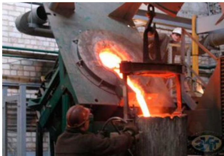
Fig. 1. Induction crucible furnace of the production frequency
