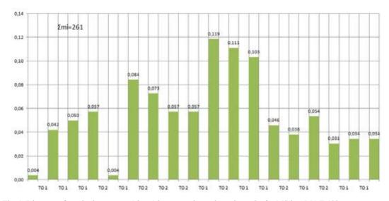
Fig. 1. Diagram of particular current (alarm) between planned repair works for MS bus MAZ-103
