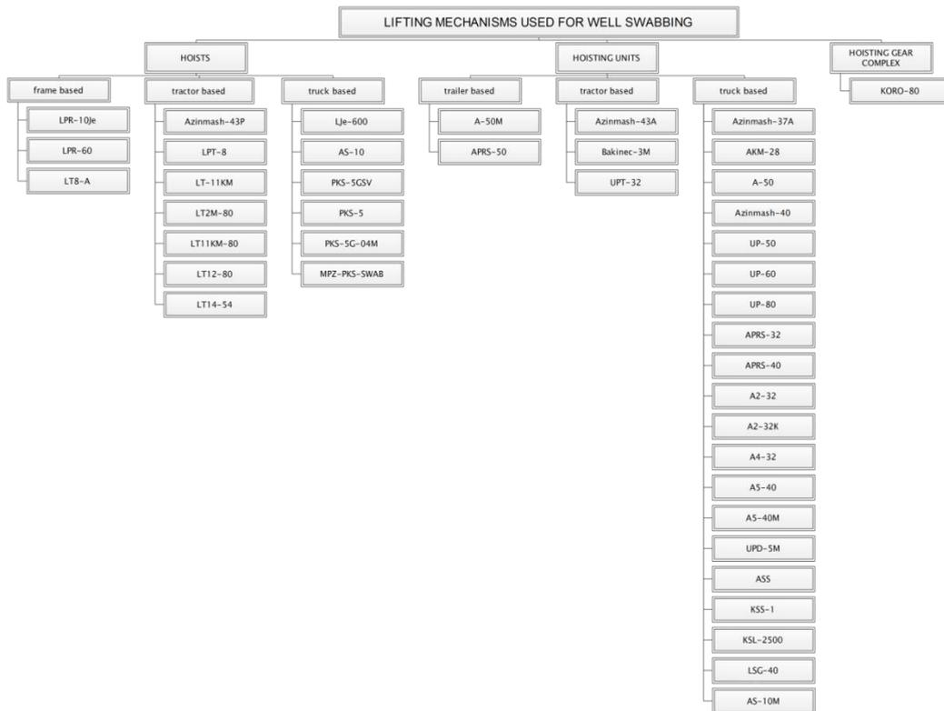
Fig. 1. Classification of lifting mechanisms used for well swabbing
