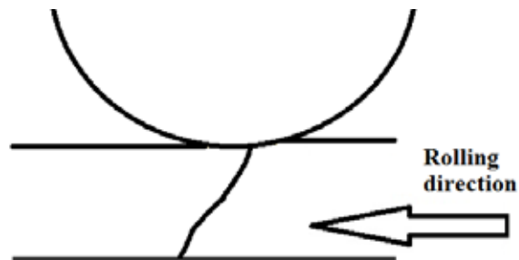
Fig. 2. Neutral section position during high section ingot rolling
