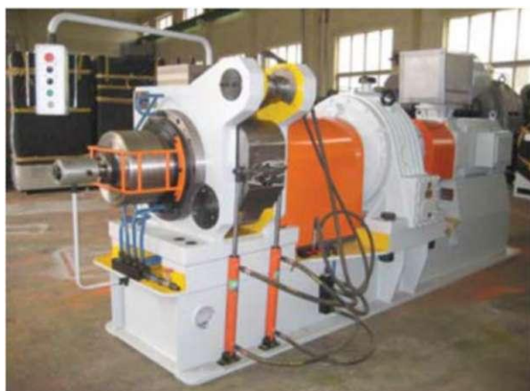
Figure-5. Overview of the Conform installation by Dalian Conform Technical Co., Ltd [6].
