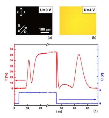
Figure 3. Optical textures of the LC cell based on the MBBA-5CB mixture ( $\Delta\epsilon=0$ ) doped with CTAB in the initial state (a) and under the dc electric field 4 V (b); the square-wave optical response of the LC cell (the top curve) placed between the crossed polarizers and electric 4 V pulse (the bottom curve) (c). The polarizer directions are shown by the double arrows.  $\mathbf{R}_1$  and  $\mathbf{R}_2$  are rubbing directions of the top and bottom substrates, respectively.
