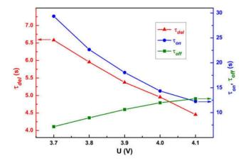
Figure 4. Delay time  $\tau_{del}$  (left axis), turn-on time  $\tau_{on}$  and turn-off time  $\tau_{off}$  (right axis) depending on the control voltage for the LC cell based on the MBBA-5CB mixture ( $\Delta\epsilon = 0$ ) doped with CTAB.
