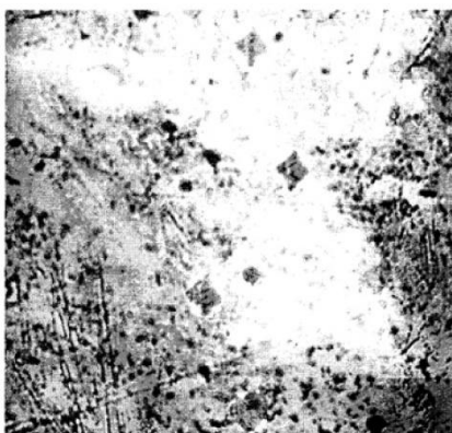
Fig. 5. Measurements of the microhardness on the cross section of the coating deposited at the substrate temperature T_k = 650 °C (magnification, \times 630 ).
