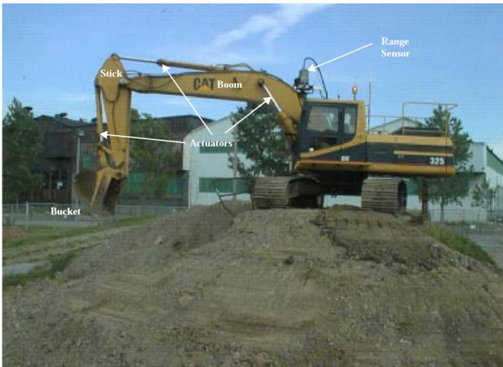
Figure 2: A side view of the Autonomous Loading System (ALS). The ALS system is a commercially available 25 ton excavator that has been outfitted with a suite of sensors and on-board computing for the purpose of automation.
