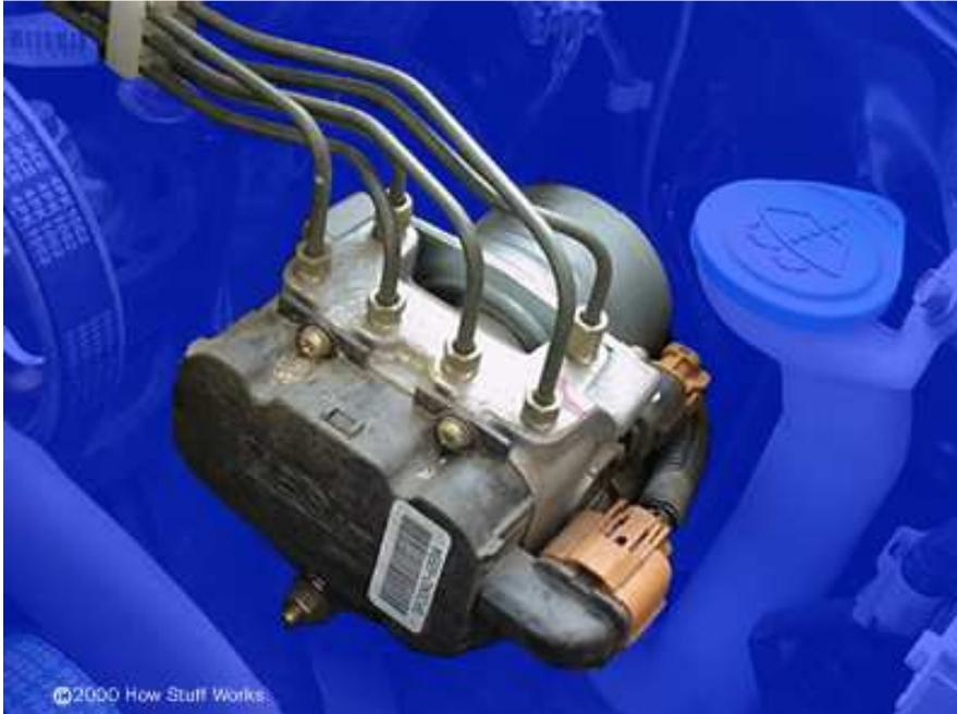
Anti-lock brake pump and valves
