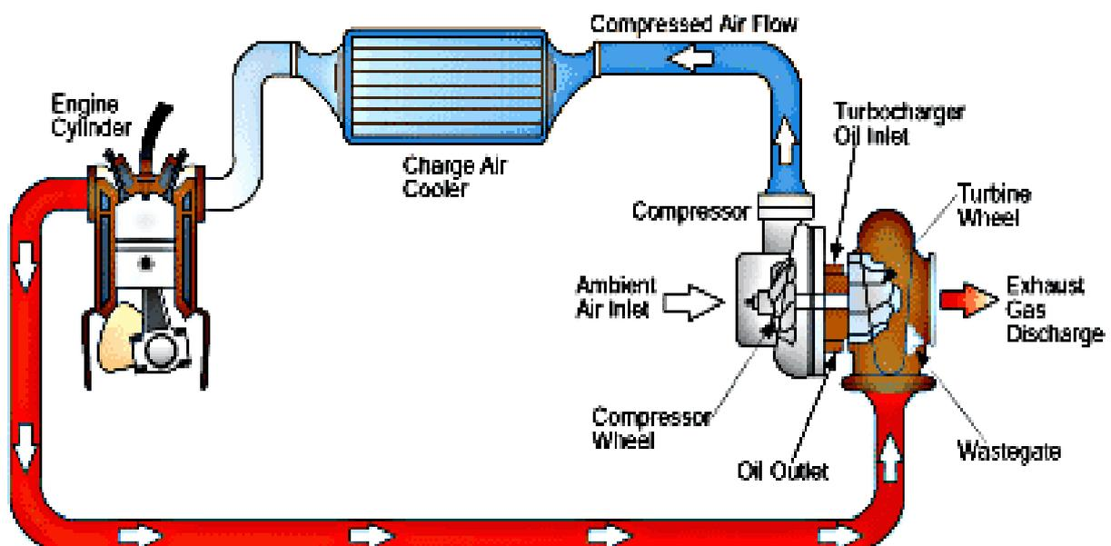
The turbocharger is bolted to the exhaust manifold of the engine. The exhaust from the cylinders spins the turbine, which works like a gas turbine engine. The turbine is connected
