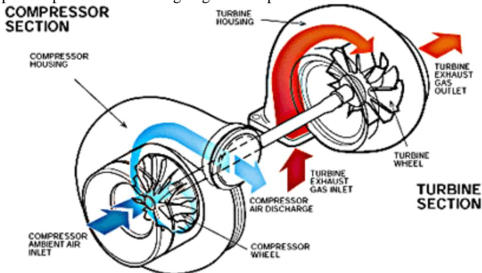
The exhaust from the cylinders passes through the turbine blades, causing the turbine to spin. The more exhaust that goes through the blades, the faster they spin.
