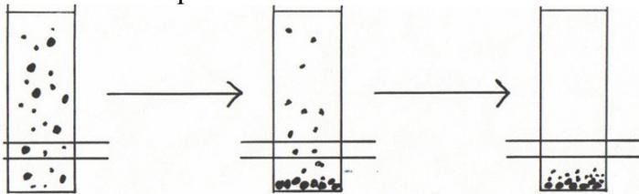
Figure 1 - Integral Sedimentation Method
