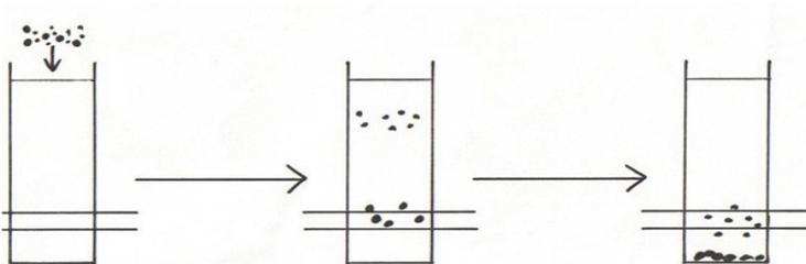
Figure 1. Integral and Differential Sedimentation Method
