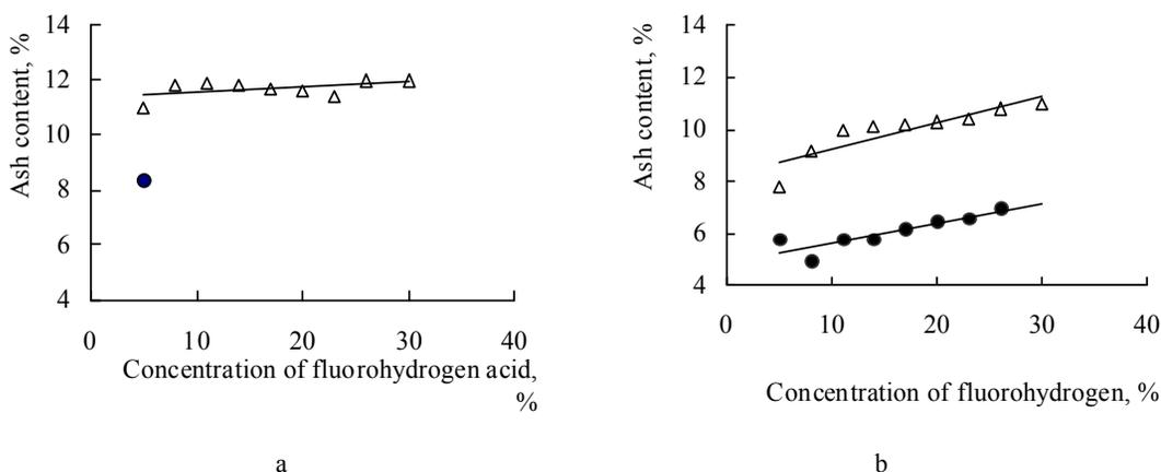
Fig. 6. Dependence of the ash content of non-activated graphite and activated graphite GLS-3 (N) on the concentration and temperature of the fluorohydrogen acid: *a* – initial graphite; *b* – activated graphite;  $\Delta$  – without heating;  $\bullet$  – with heating
