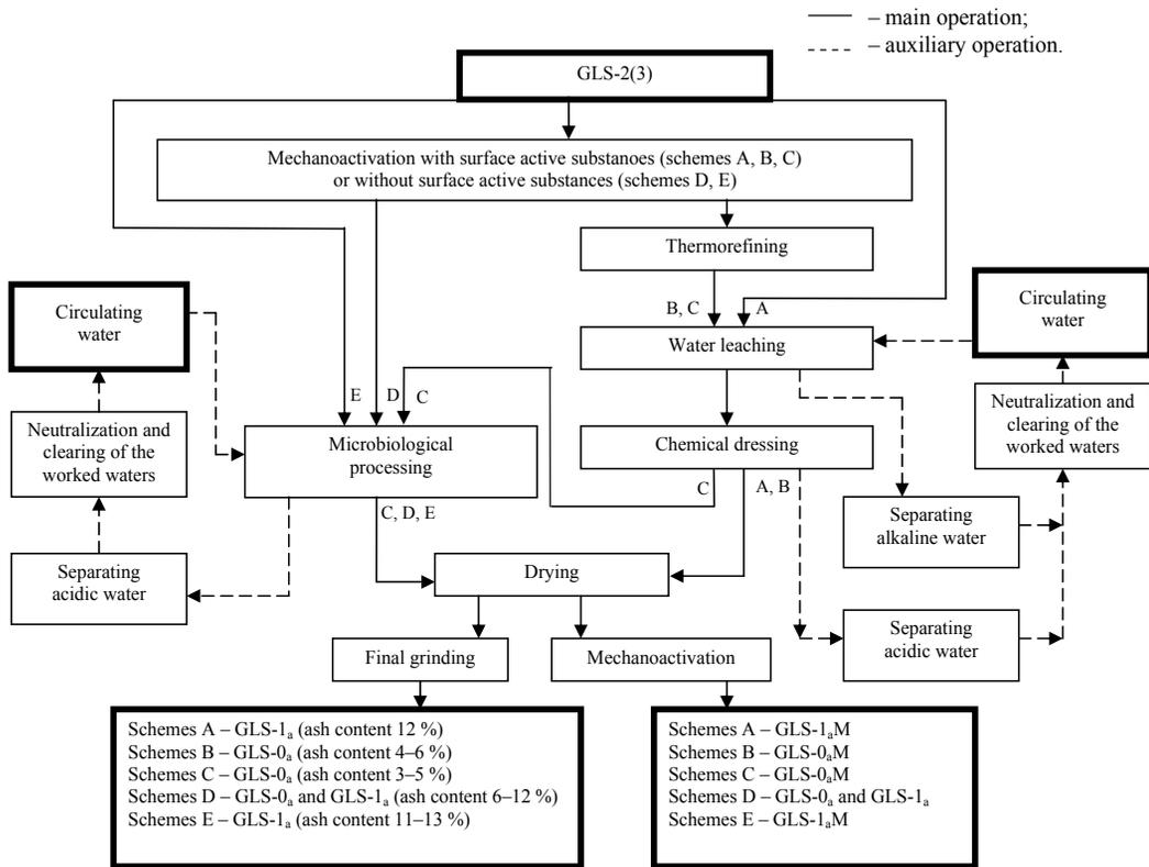
Fig. 16. Schemes of dressing cryptocrystalline graphites
