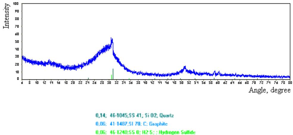
Fig. 10. Phase composition of the processed Noginsk graphite GLS-0 (N)<sub>a</sub>
