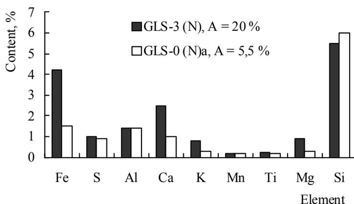
Fig. 7. Element composition of graphite GLS-3 (N) (A – ash content)
