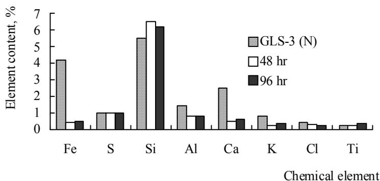
Fig. 15. Dependence of the element composition of graphite GLS-0 (N)<sub>a</sub> on the processing time
