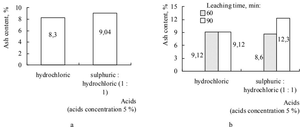
Fig. 5. Dependence of the ash content of the graphite GLS-3 (N) on the chemical concentration parameters: *a* – the mixture «graphite–soda ash» (the time of leaching with hot water is 60 min); *b* – activated mixture «graphite–soda ash» (the time of leaching with not water is 60 and 90 min)
