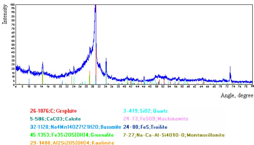
Fig. 9. Phase composition of graphite GLS-3 (N)
