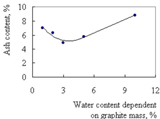
Fig. 4. Dependence of the ash content of graphite GLS-3 (N) on water content in the mixture «graphite–soda ash – water»
