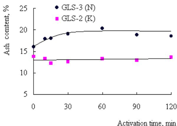
Fig. 1. Dependence of graphite ash content for GLS-3 (N) and GLS-2 (K) on graphite activation time
