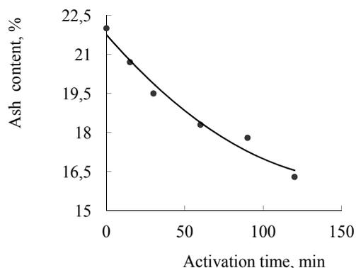
Fig. 2. Dependence of graphite ash content for GLS-3 (N) on the time of graphite activation together with soda ash
