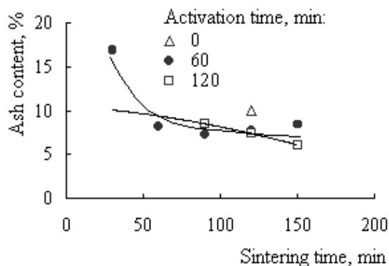
Fig. 3. Dependence of the ash content of graphite GLS-3 (N) on the activation time and sintering time (sintering temperature is 860 °C)
