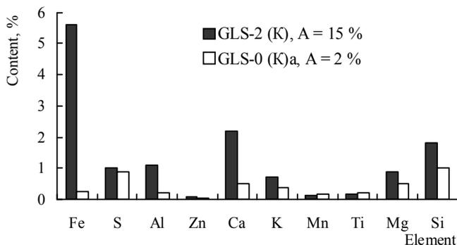
Fig. 8. Element composition of graphite GLS-2 (K) (A – ash content)
