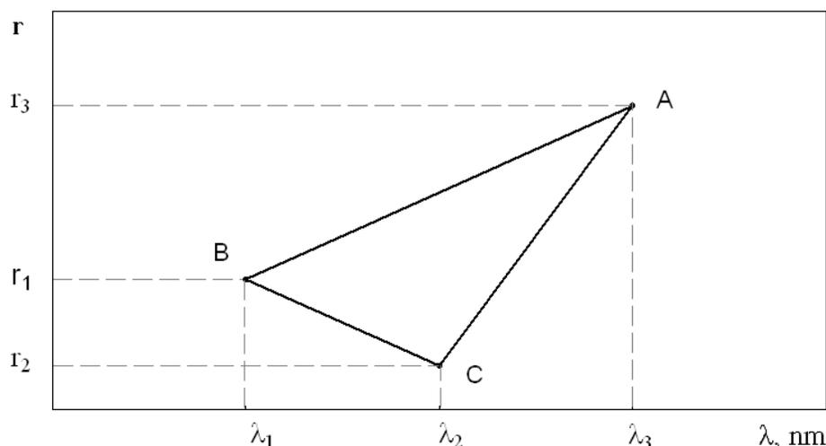
Fig. 3. A schematic representation of the triangle with vertices  $(\lambda_i, r_i)$  used to calculate CPSP
