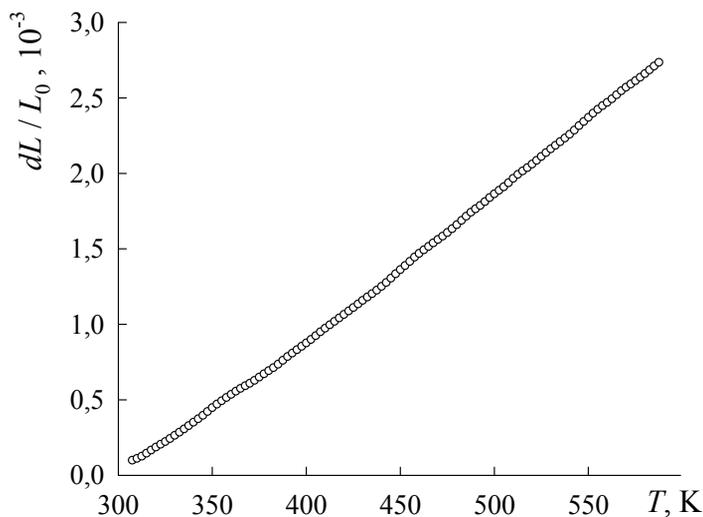
Fig. 2. Influence of the temperature on the relative length extension ( $dL/L_0$ ) of the  $\text{PbGeO}_3$  glass
