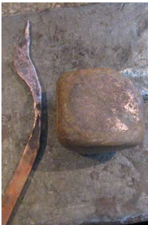
Fig. 7. Copper billet and smoother for its cold treatment
