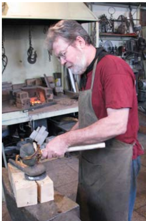
Fig. 1. Process of experimental smithery of hot metal with use of stone tools
