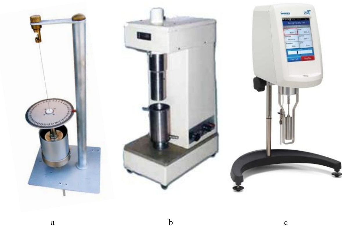
Figure 1. Apparatus for measuring the static shear stress, yield point and plastic viscosity of the drilling fluid: SNS-3 (a); VSN-3 (b); Brookfield rotational viscometer (c).
