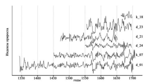
Fig. 1. Example of cross-dating of the samples, taken from the construction No. 1a. *Note: samples numeration is given according to table No.1*
