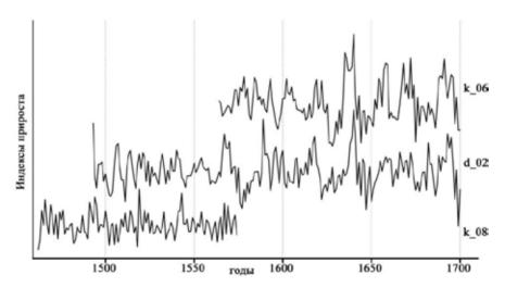
Fig. 2. Example of cross-dating of the samples, taken from the construction No. 2. *Note: samples numeration is given according to table No. 1*
