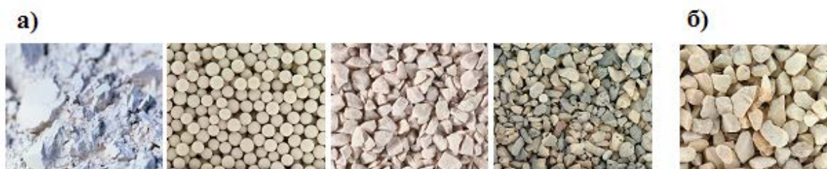
a) – the size of grains of a sorbent, b) – ore, for production of a sorbent
