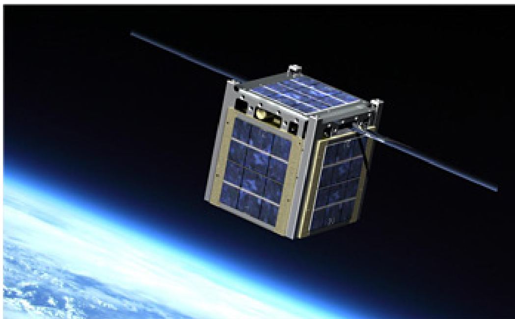
Pic. 1 –Cubesat, type of miniaturized satellite for space research that is made up of multiples cubic units
