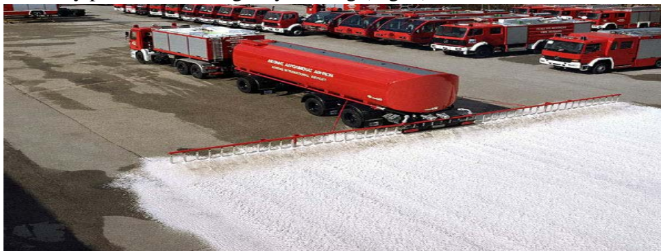
Figure 2. Spreading of fire suppression foam layer on the airport runway
