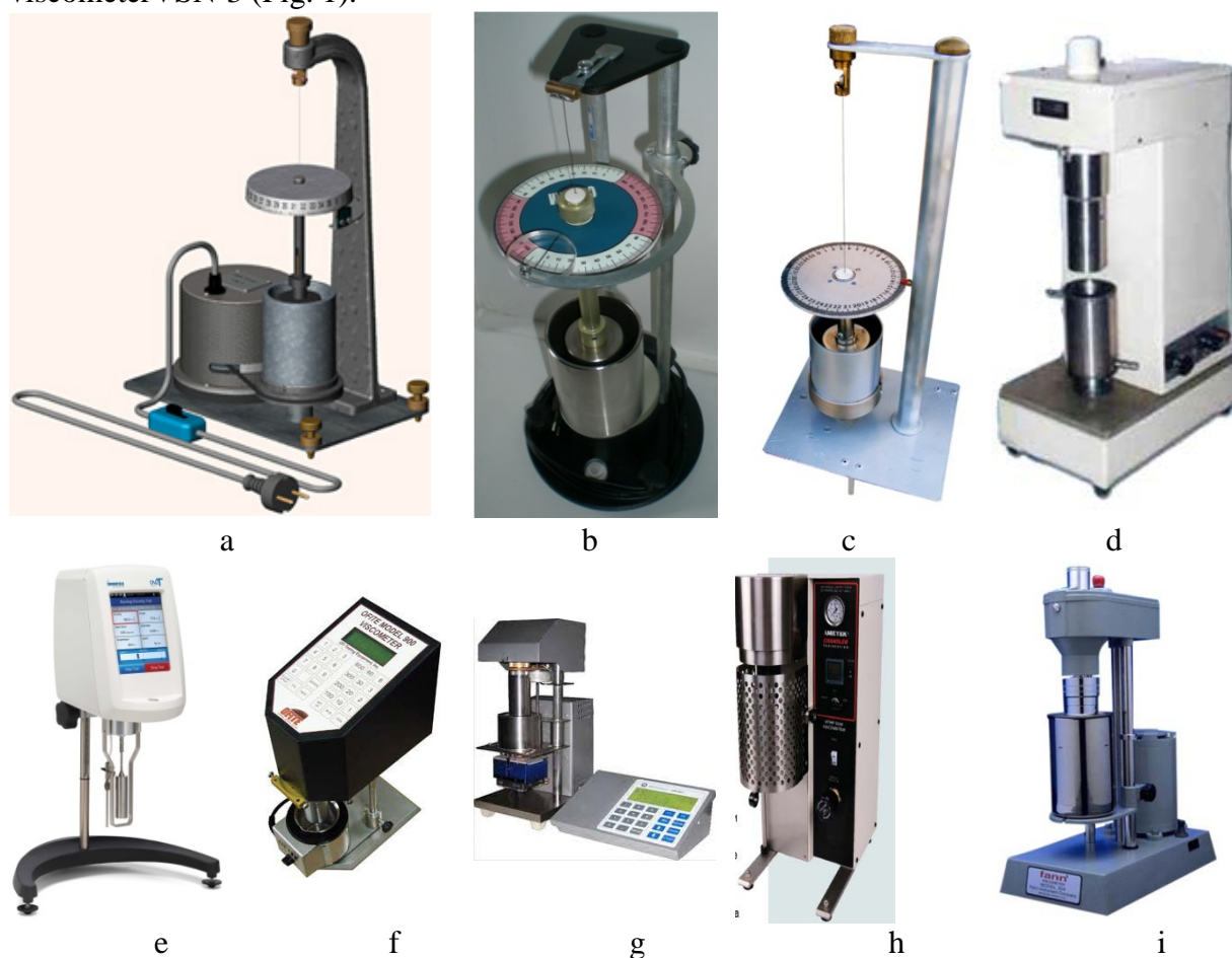
Figure 1. Apparatus for measuring static shear stress, yield point and plastic viscosity of the drilling fluid: a - SNS-2; b - SNS-2M; c - SNS-3; d - VSN-3; e - Brookfield rotational viscometer series DV2T; f - rotational viscometer series OFITE; g - rotational viscometer series ZIM; h - rotational viscometer series CHANDLER; i - rotational viscometer series FANN.
