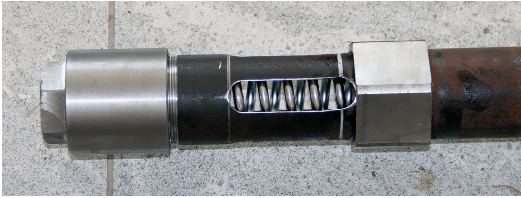
Figure 3. The hydrodynamic well generator of spring-valve-type
