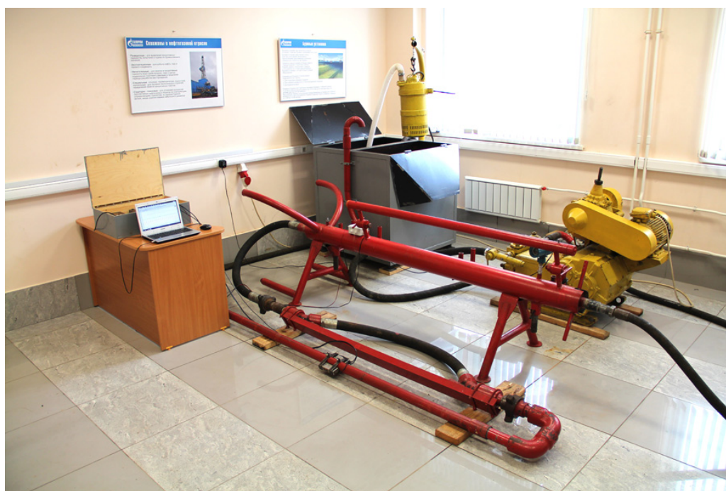
Figure 1. The laboratory stand for the research of the HWG
