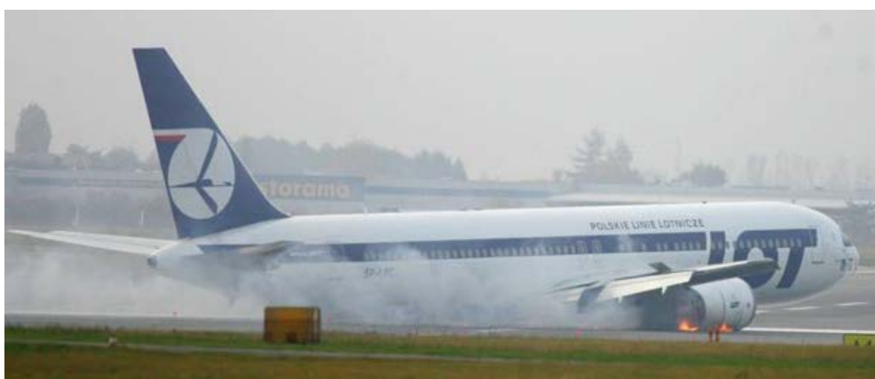
Figure 1. A passanger jet made an emergency landing on a protective layer of foam
